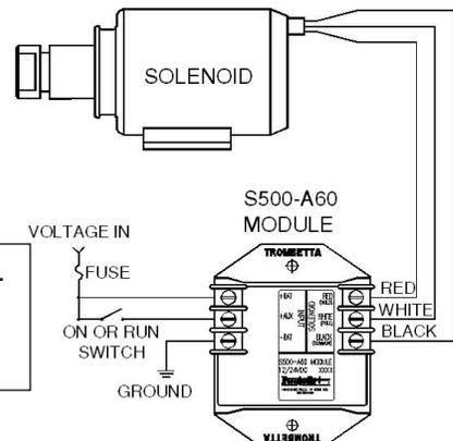
3. S500-A5 & A50 Modules - After making the final wiring check, energize the solenoid hold coil by turning the switch to the On+ position and manually push the solenoid plunger to the seated position. The plunger should remain seated.
