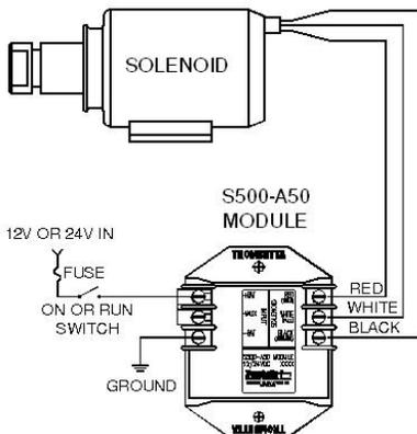
\*\*\* Note when using an S500-A50 or S500-A60 module all of the solenoid connections must connect to the module as shown. **Do not** connect any of the solenoid leads to another ground point in the system.
