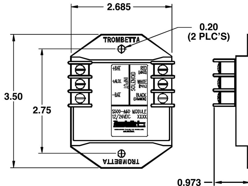
**NOTE: When using a S500-A60 module all of the solenoid connections must connect to the module as shown.**
