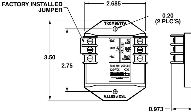
**NOTE: When using a S500-A50 module all of the solenoid connections must connect to the module as shown.**
